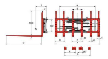
with independent sideshift - with bolt-on forks, Pallet handling lengthwise 800 x 1.200 mm for 4 or 6 pallets - 2 hydraulic functions
