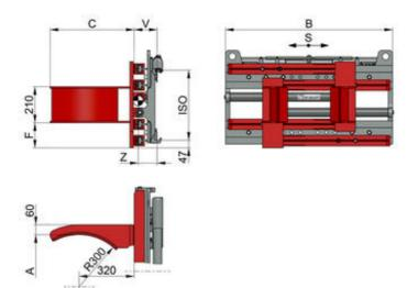
with independent sideshift - for cylindrical steel drums - 2 hydraulic functions, This Drum Clamp can transport 1 or 2 drums palletless and safely.
