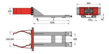
slip-on-fork version, arms coated with Remagrip - for cylindrical steel drums and garbage bins - without rotation - 1 hydraulic function
