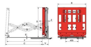
Push-Pull with sheet saver T145SA, slip-on-fork version - 1 hydraulic function - and built-in solenoid valve with accessory kit
