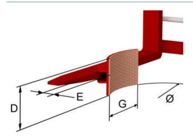
slip-on version, for handling of cylindrical steel drums) - rubber coated
